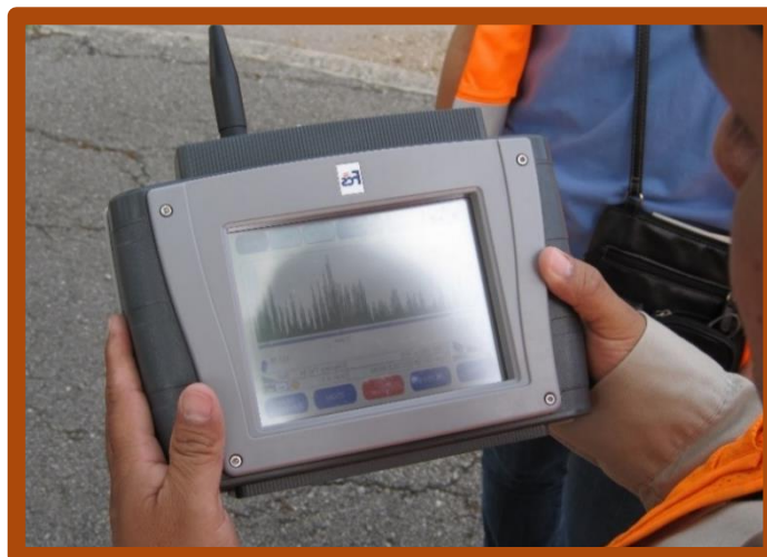
Figure 3-6 Leak Detection Equipment
