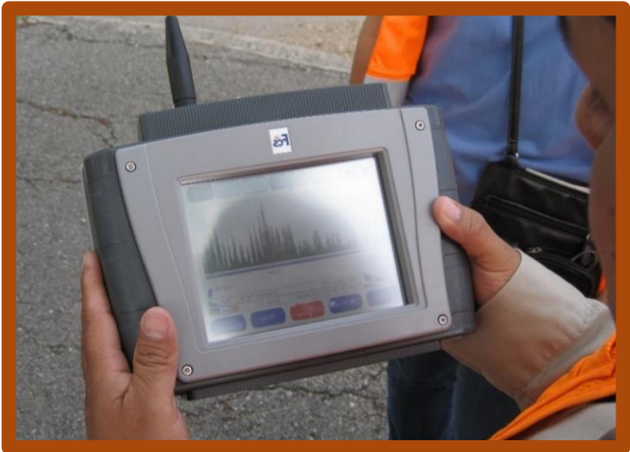
Figure 3-6 Leak Detection Equipment
