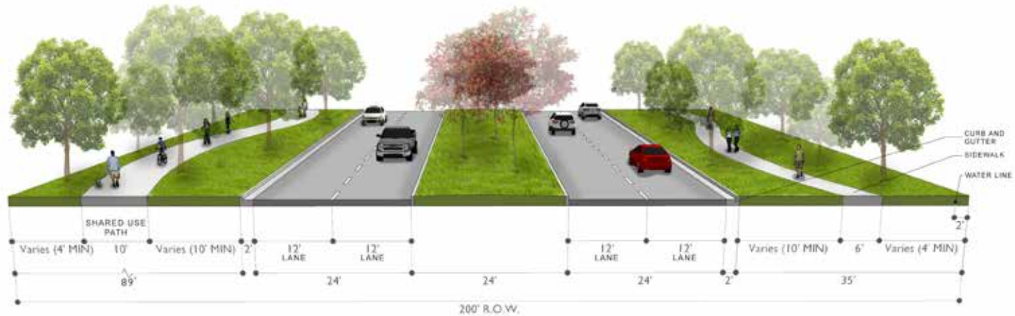
Figure 8-10 Cross Sections – Parkway
