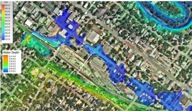
Existing 100-year storm flooding
