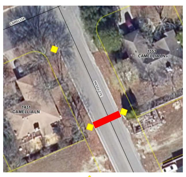
Speed Hump Proposed Location Speed Hump Signs Proposed Location
