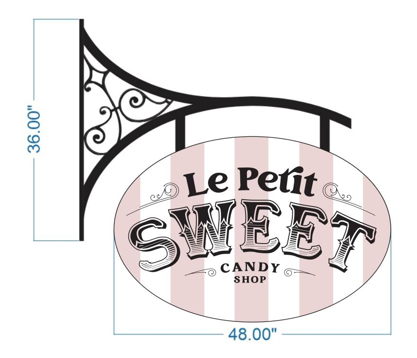
DESCRIPTION: STEEL/SLUMINUM CONSTRUCTION SIGN BLADE STYLE STEEL MOUNTING BRACKET AND HANGERS **AETHER**
