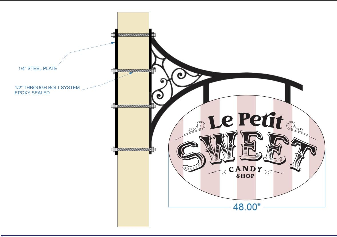
**DESCRIPTION:** STEEL/SLUMINUM CONSTRUCTION SIGN BLADE STYLE STEEL MOUNTING BRACKET AND HANGERS **AETHER**
