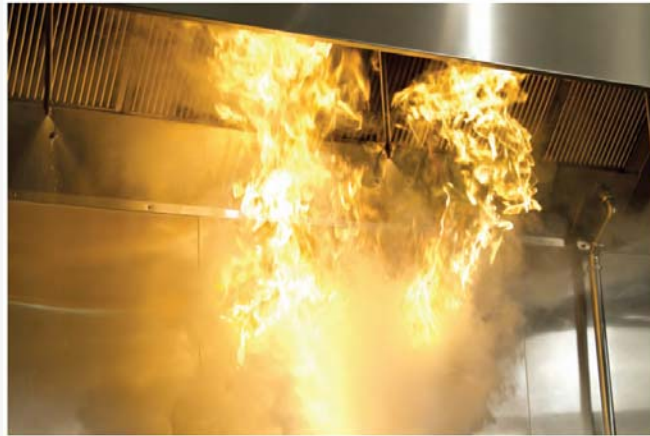
Automatic water mist system protecting commercial cooking operation
