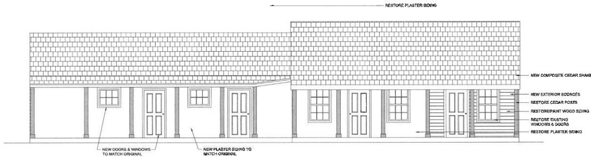
01 PROPOSED ELEVATION Front SCALE: 1/4" = 1'-0"
